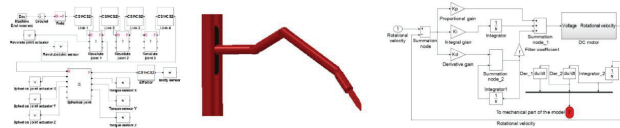
Fig.1. Mechanical model of the medical robot and steering system with DC motor in Simulink
